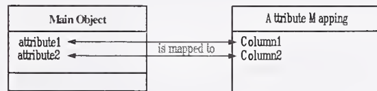
Fig. 2 Mapping attributes of an XML Element to the columns of its corresponding RDB table
